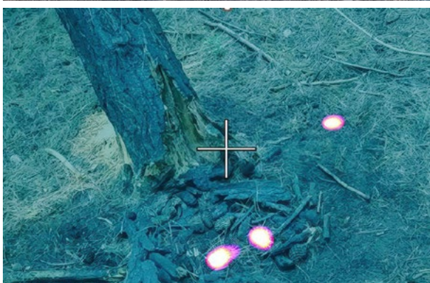
Naked eye and thermal camera view of buried heating pads
