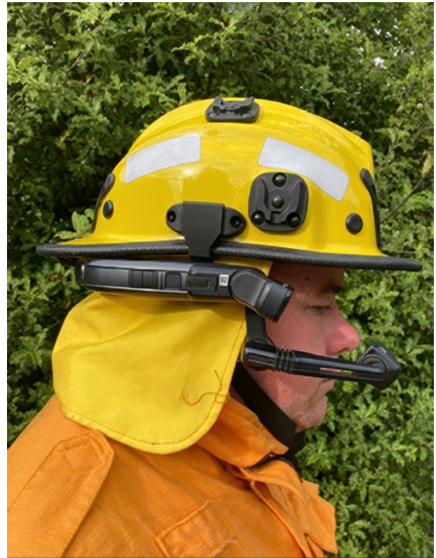
Camera attached to a New Zealand fire helmet
