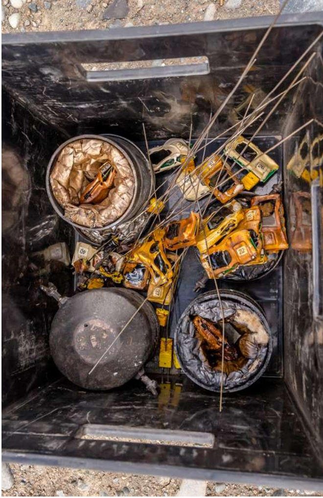
Data loggers recording the rate of fire spread succumb to the heat despite being housed in well-insulated, low-to-the-ground, capsules. Photo: Scion
