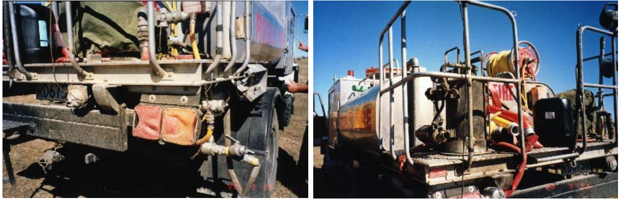
Figure 7 (a) & (b). Damage to the DCC fire appliance, including tail lights, foam proportioner, pump cover and rubber hose fittings.
