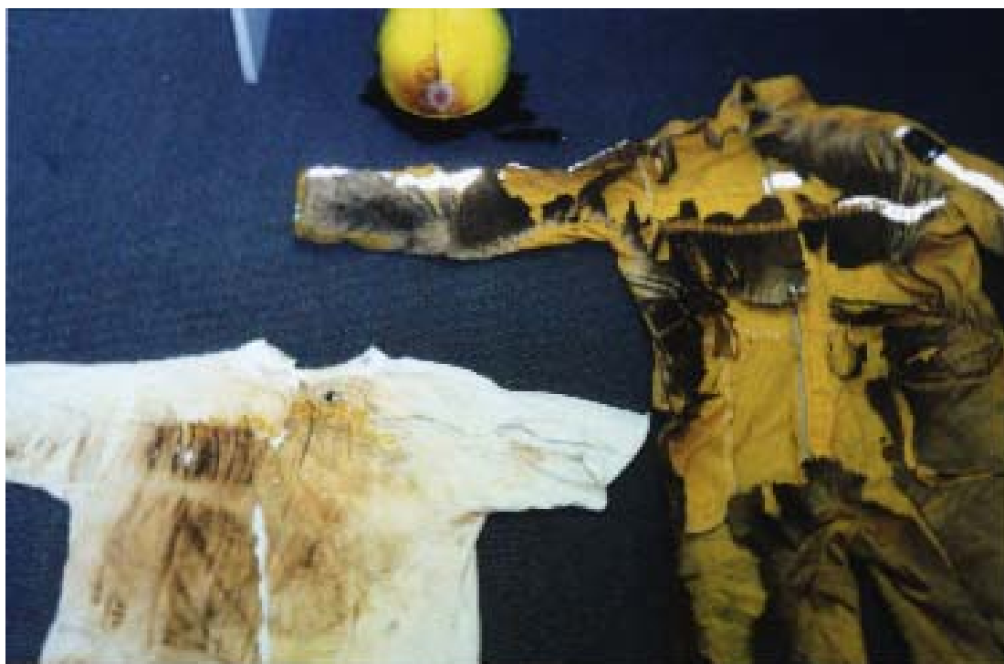
Figure 29. Damage to personal protective clothing from Firefighter C (who received the most serious burn injuries), including Nomex coveralls, cotton T-shirt and fibreglass helmet.
