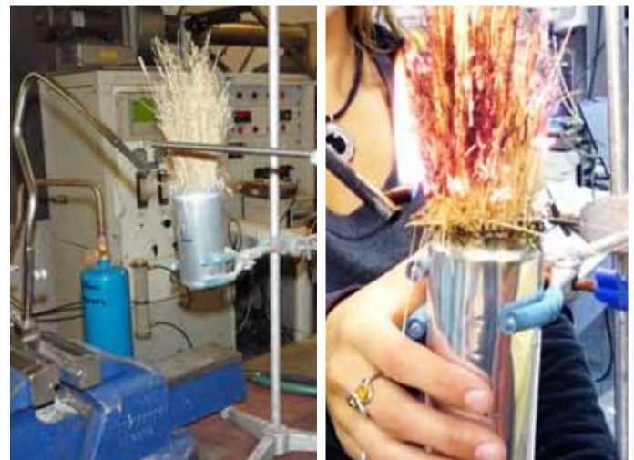
Figure 5. Open flame experimental set-up (left), and exotic grass sample ignition (right).
