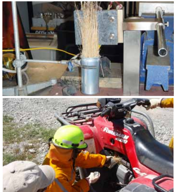
Figure 1. Grass sample held in contact with the copper hot plate in vertical orientation (top) and ignition testing of an exotic sample at the manifold of an ATV (bottom).
