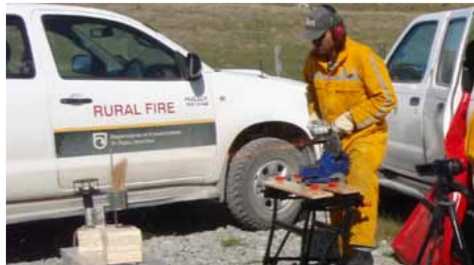
Figure 3. Metal sparks experimental set-up in the laboratory (top) and field (bottom).
