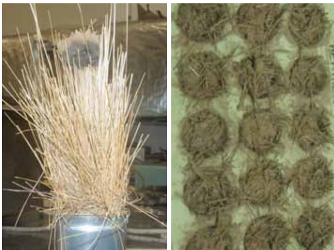
Figure 4. A tussock sample with a disk placed on top (left), and organic embers in moulds (right).
